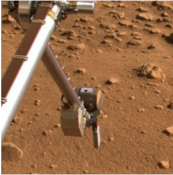
Fig. 3-1. NASA's Phoenix Mars Lander's Robotic Arm with its thermal and electrical conductivity probe, at the lower right, pointing toward the Martian soil (July 14, 2008). Photo credit: NASA/JPL ( link ).
