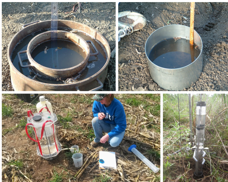
Fig. 6-5. Photographs of a double-ring infiltrometer (top left; Source: Wikipedia, public domain), single-ring infiltrometer (top right; Source: Wikipedia, public domain), mini-disk tension infiltrometer (bottom right), and sprinkle infiltrometer (bottom left, Source: Iowa Learning Farms, used by permission).
