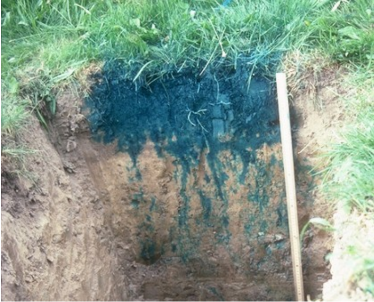
Fig. 9-3. Preferential flow in a soil near Ithaca, New York, revealed by a blue dye applied with infiltrating water. Source: http://soilandwater.bee.cornell.edu/research/pfweb/educators/intro/macroflow.htm
