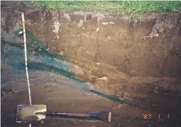
Fig. 9-5. Blue dye highlights the preferential flow caused by a sloping coarse-textured soil layer at a field site in New York. Source: http://soilandwater.bee.cornell.edu/Research/pfweb/educators/intro/img_funnel.htm
