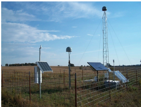
Fig. 3-2. Sensors at the Marena, Oklahoma, In Situ Sensor Testbed (MOISST) site including sensors for the cosmic-ray neutron method (white box on right) and GPS reflectometry method (gray domes on masts), as well as numerous types of below ground soil water content sensors.
