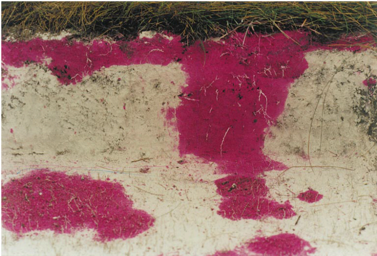
Fig. 9-4. A dye staining experiment reveals preferential flow paths in a hydrophobic sand dune in the Netherlands. Reproduced from Dekker and Ritsema (2000).
