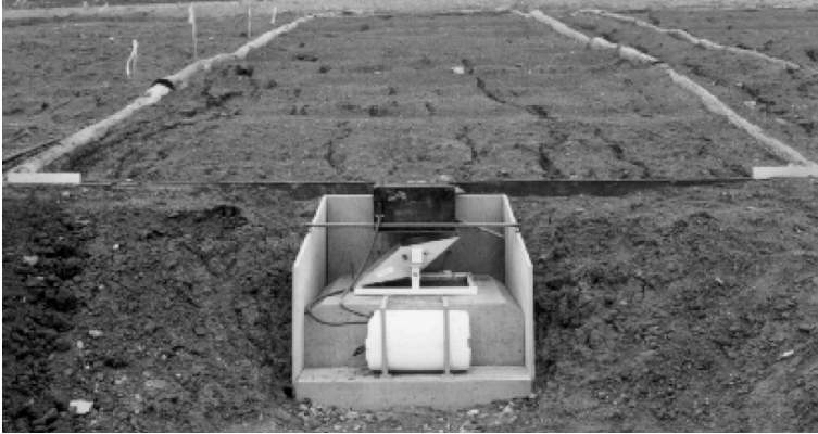
Fig. 6-6. Photograph of a 20-m long by 5- m wide runoff plot in Queensland, Australia. This plot is equipped with a tipping bucket device to measure runoff. Reproduced from Carroll et al. (2000).
