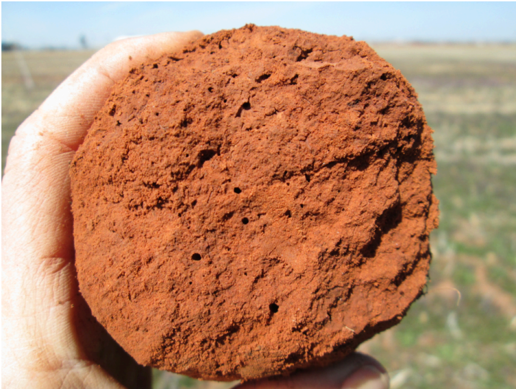
Fig. 4-1. Macropores in a sub-soil core pulled from an alluvial soil along the south side of the Washita River near Chickasha, Oklahoma.
