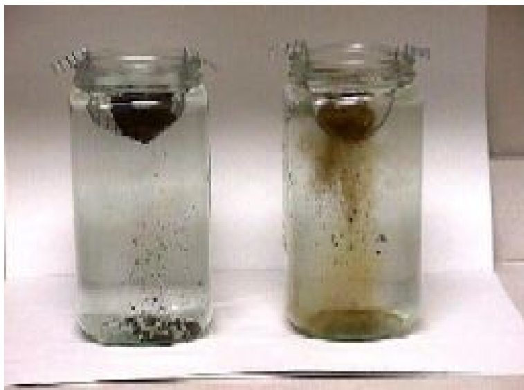
Fig. 2 9. Simple method for demonstrating aggregate stability. Photo credit: USDA-NRCS ( link ).
