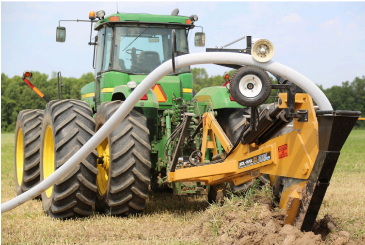
Fig. 8-5. Tractor and tile plow installing plastic drainage tile in cropland. Source: Ag Leader Technology ( link ).
